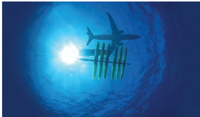
Liquid Robotics' Wave Glider floats on the surface of the ocean, but it's propelled by a wave-powered undersea glider. (Liquid Robotics Photo)
