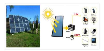
Fig. 87: Extended PV solar home system [6]
