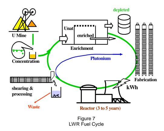
The typical PWR fuel cycle is made up of the following stages:
