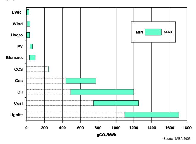
Figure 12 Life-cycle emissions of GHG (in equivalent g CO<sub>2</sub>) to generate 1 kilowatt-hour of electricity.
