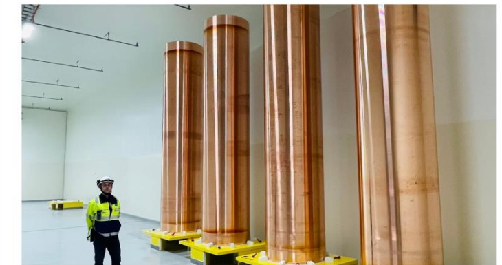
Four of the test spent fuel canisters used for the encapsulation plant trial run. Image courtesy Posiva.
