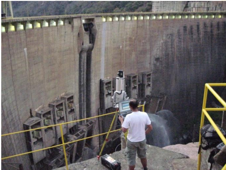
Advanced engineering technologies using laser scanning at for monitoring the Cahorra Bassa Dam, Mozambique, one of the largest in the world. © Antonio Berberan, Eliane Portela and João Boavida
