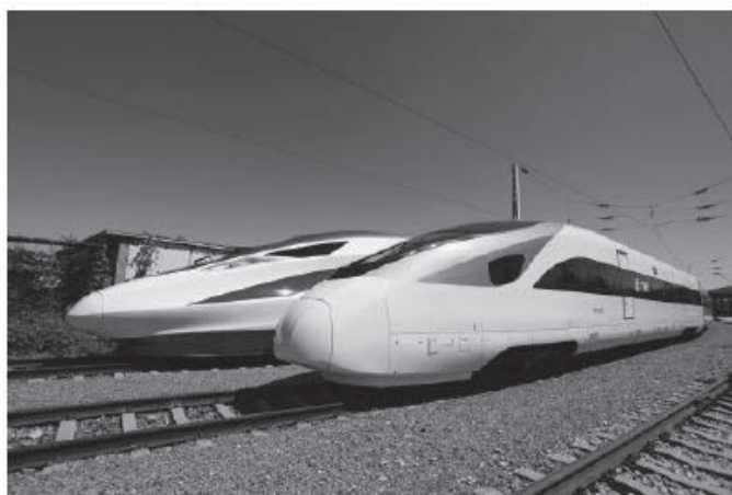
Standard EMU in China (4M4T, with the maximum operating speed of 350km/h and the maximum axle load of 17t)
