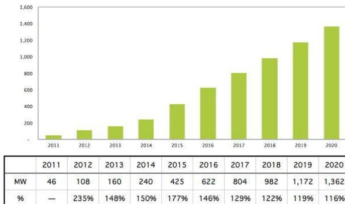
Fig. 33: Yearly installed capacity of high concentration PV systems [9]
