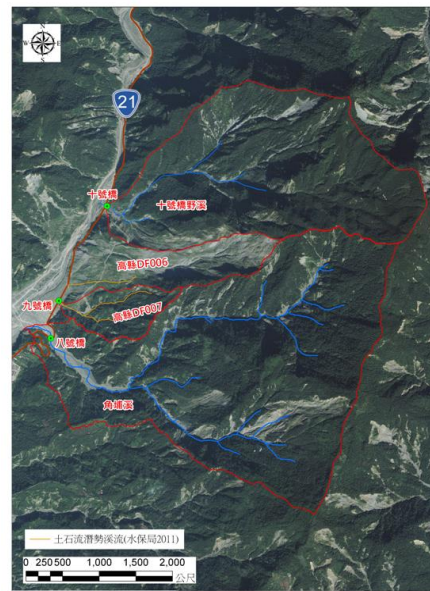
Figure 12. The stand of debris flows after Typhoon Morakot
