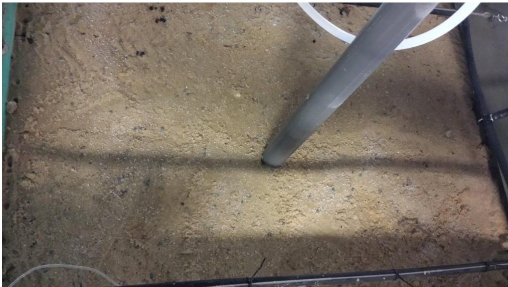
Figure 105 – Tracer grains on the top of the soil from the physical (sandbox) model, Experiment 2
