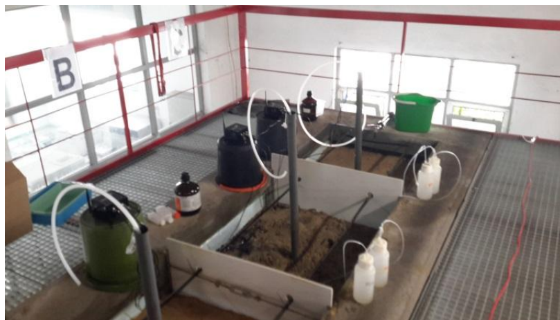
Figure 103 – In situ monitoring devices, both for the saturated and vadose zones
